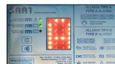
If the alarms are type "B" (**fault** alarms) the LED matrix lights forming the letter B.
