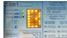
This is also a battery to keep active alarms in the absence of power supply and a piezoresistive buzzer for the active alarms signalization.
